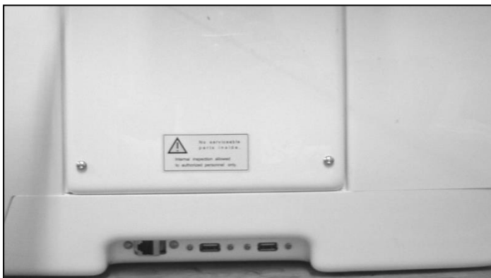
Fig. 6 – USB and Ethernet connectors (left) / power inlet and main switch (right)
