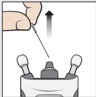
Remove the probe and place it back into the probe container.
