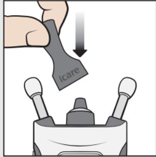
Place the probe applicator over the probe base.
