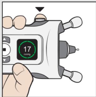
After a successful measurement, press the Measure button (▶) once and repeat the measurement on your other eye.
