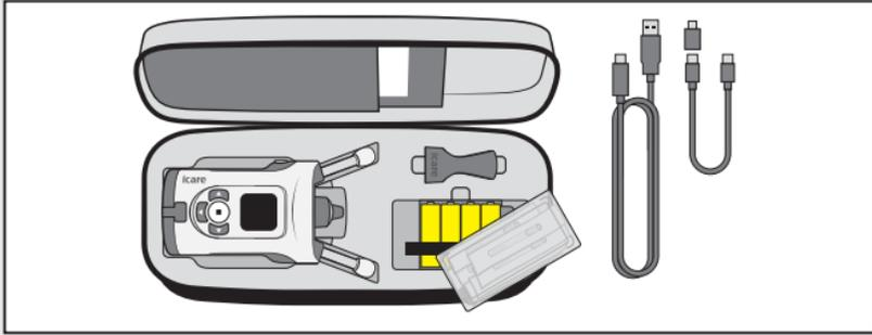
The batteries are in the tonometer carrying case under the box of probes.
