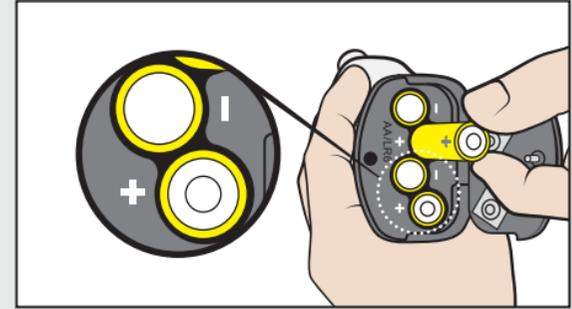
Insert the batteries, and close the cover.
