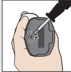
Open the battery cover with the screwdriver.
