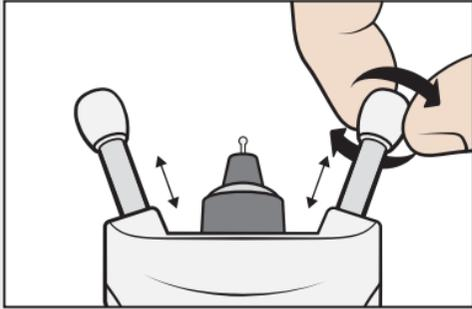
Before the measurement, adjust the forehead and cheek supports to the correct length. Start with the supports at the maximum length.
