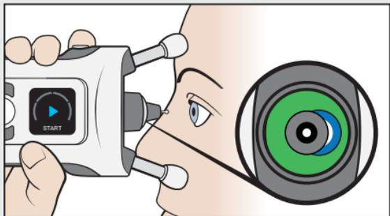
If the rings are not symmetrical, the probe does not point perpendicularly to the center of your eye. Correct the position of the tonometer.
