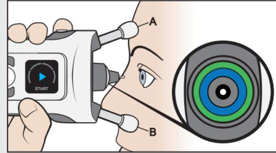
Place the tonometer against your face and look into the probe base. The probe points perpendicularly to the center of your eye when the blue and green rings in the probe base are symmetrical.
