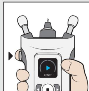
A measurement sequence consists of six measurements.
